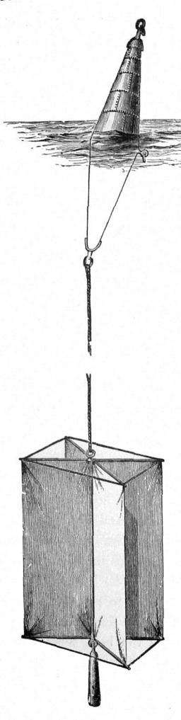
Fig. 89.—The Current-drag and Watch-buoy.
